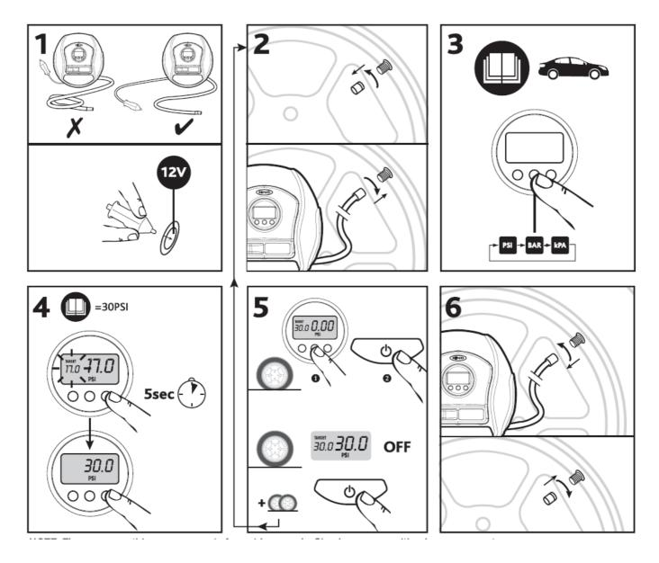
**NOTE**: The gauge on this compressor is for guidance only. Check pressure with a known accurate gauge. The compressor can be used without the engine running but this will drain the power from the battery.
