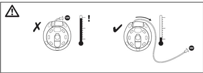
Please ensure to fully unwind the power cable before use to avoid overheating.
