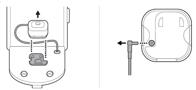
Pull the tabs on the side of your sensor to remove the back cover.
