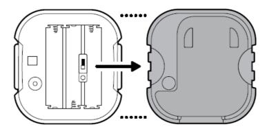
Keep the switch in the battery compartment flipped toward the octagon marking.
