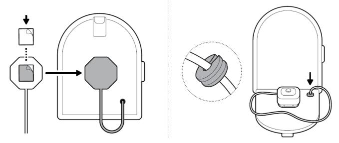
11. Manage the cable with the included cable management system.
