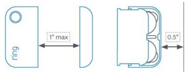
Ensure no more than 1 inch (25.4 mm) between sensor and magnet when the door or window is dosed. Leave at least a 1/2 inch (12.7 mm) space so you can open the battery compartment.
