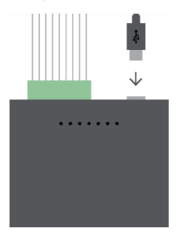
If you mounted your device outside the call box, plug it into an outlet using the included micro USB cable and DC power brick.
