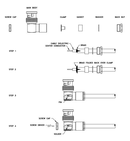
**Step 1:** Cut end of cable evenly. Strip cable to dimensions shown in catalog or on outline drawing. All cuts are to be clean and square. Do not nick braid or center conductor when cutting. Slide back nut, washer and gasket onto cable. Comb braid for assembly of clamp.
