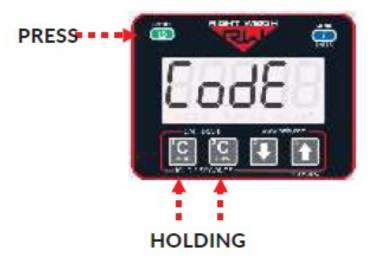
Press the MENU button and "——" will display on the screen. Enter the previous PIN code. If the code entered is correct, the display will show "Good
