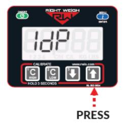
• The numbers on the images indicate the axle groups that will be displayed on the gauge. To cycle through the axle group on the gauge, press the MENU button
