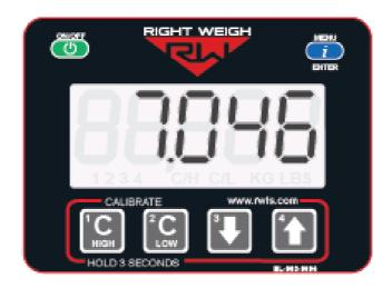
• In this example, strain sensor A is out of range and needs to be manually adjusted until it is between 6.500 and 7.500.
