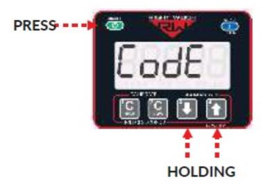
Press the MENU button and "00000" will display on the screen. Enter a 5 digit PIN code using the 1, 2, 3, and 4 buttons. Press the MENU button again to save the code. \*\*If the display shows "——", then there is already a code set
