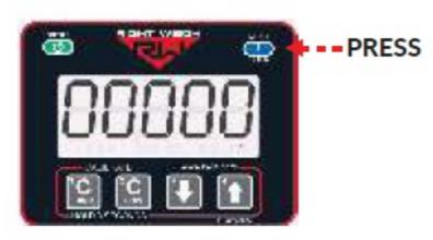
With the gauge off, press and hold both the C LOW and C HIGH buttons, then press the ON/OFF button. Release all three buttons. The gauge will display "CodE
