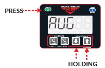
• Press the UP arrow button to cycle through the operating modes. To 1 2 3 4 C/H C/L KG LBS confirm your selection, turn the scale off by pressing the ON/OFF button.
