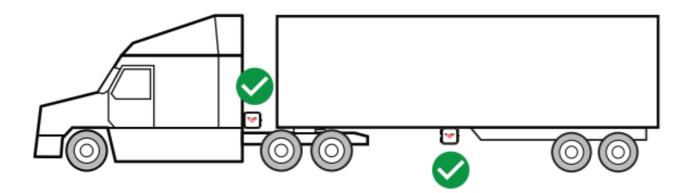
DO NOT mount the scale directly to the chassis or any other main beam unless it is approved by the vehicle manufacturer. Doing so may void the warranty with the vehicle manufacturer.
