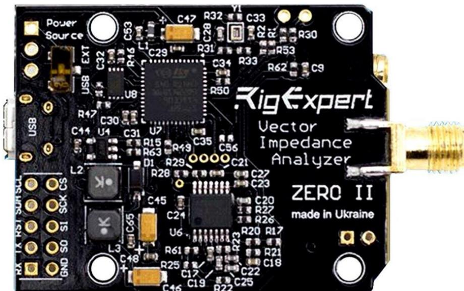
The Zeroll in measurement mode supports communication with the host controller via SPI, I2C, UART. I2C interface use 7-bit slave address 0x5B. The firmware is updated via the USB interface using the RigExpert Flash Tool utility. Commands supported by SPI, I2C, UART interfaces:
