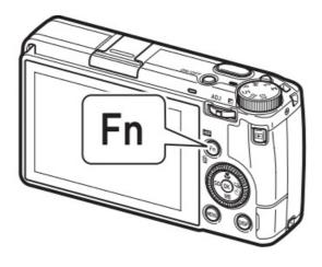
The function of FN can be changed in [Fn Button Setting] of the C2 menu. [HDF] is set by default.
