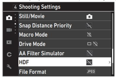
[HDF] is supported by [Memory] of the D2 menu. The [HDF] setting is retained even after the camera is turned OFF and back ON.
