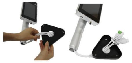
3. Pass all the data interface cables through the hole in the stand backside cover.
