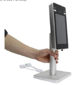
3. Connect the Ethernet and Power Cable to the Stand Base connectors.
