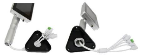
4. Connect the USB, Ethernet, and Power Cable to the Stand Base connectors.
