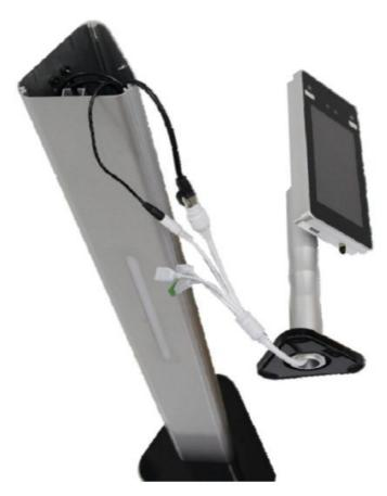
5. Screw the V3 mount into the base stand and secure it from the bottom using the helix nut provided. The mount is meant to be screwed in, not forced indirectly.
