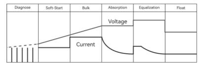
Diagnose\*- Only for Lithium battery type, subjected to the Lithium battery ini-tial voltage then determine if going to Soft-start or Bulk charge; if the Lithium battery is protected by BMS, the controller will automatically send the signal periodically to the battery terminals to activate the BMS against protection.
