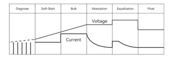
**Diagnose:** Only for Lithium battery type, subject to the Lithium battery initial voltage then determine if going to Soft-start or Bulk charge; if the Lithium battery is protected by BMS, the controller will automatically send the signal periodically to the battery terminals to activate the BMS against protection.
