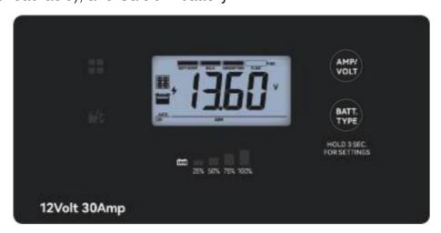
Press and hold the BATTERY TYPE BUTTON for 3 seconds to enter battery type selection mode. The selected battery type will be shown on the LCD meter. The default setting is AGM Battery, and the controller will automatically memorize your selection. LiFeP04 battery shown in LCD indicates Lithium Iron Phosphate battery, LFP battery.
