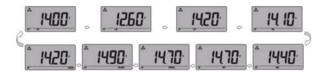
Press the AMP/VOLT button again to confirm the selected battery type (it will stay solid). Alternatively, the selection will be automatically confirmed after 3 seconds.
