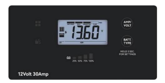
Press and hold the BAT T. TYPE button for 3 seconds to enter battery type selection mode. The selected battery type will be shown on the LCD meter.
