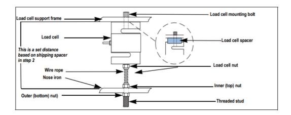
Screw the inner nut on the wire rope flush with the top of the threads. The inner nut is what is used to set the distance measured from the shipping spacer.
