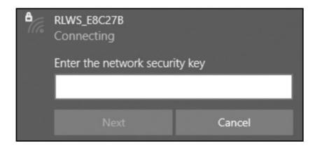
The X's in the name represent the last 6 digits of the WiFi MAC address. The serial number on the WiFi module's label is almost the same, other than the last digit being one number/character less than the WiFi MAC address. For example, if the module's serial number is "0080A3E8C27A", then the SSID would be "RLWS\_E8C27B". The MAC address is a Hexadecimal value, so the letter A follows the number 9, and this continues to F before incrementing the next most significant digit and returning to 0.
