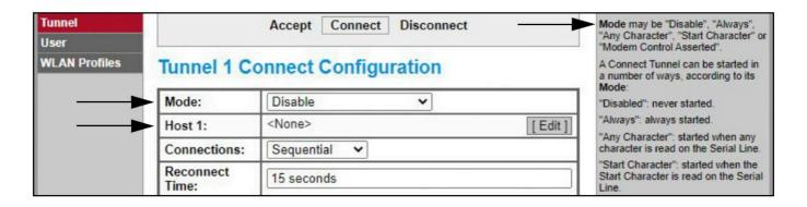
Set the Address and Port as needed to connect to the intended available server connection.
