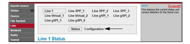
Use drop-down options to change Line 1 Configuration settings as needed to match the product's serial port settings.
