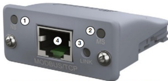
Figure 2-5. Modbus TCP Status LED Module
