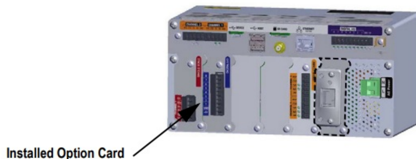
Figure 2-4. Installed Interface Option Card
