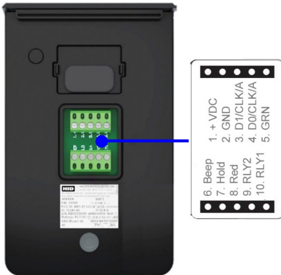
Figure 6. HID Reader Terminal Block Pinout
