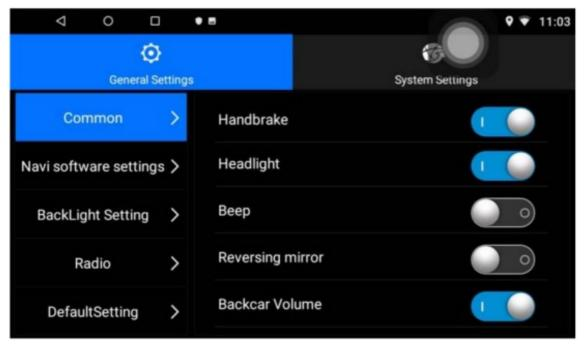
Handbrake: press this on, then the device will not allow drivers to watch video during driving due to safety reason Headlight: press this on, the unit will detect the light signal from the orange wire named "+ill". If the wire is connected to the car lamp, then the unit button light will auto adjust according to the car lamp on/off Beep: press this on to have the beep sound when you press the touch screen
