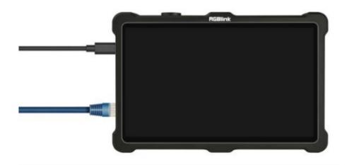
6. After connection, press the power switch on the top panel to open the device.
