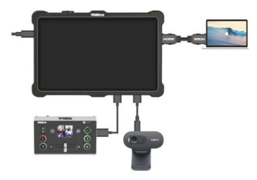
3. Connect monitor to HDMI OUT interface to preview the input and output.
