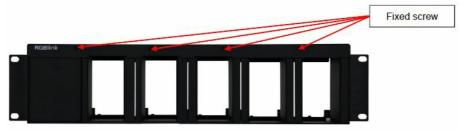
2. Install the small converters to the slots, as shown in the figure:
