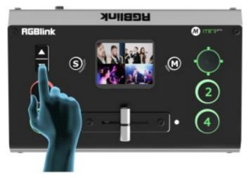
Press button S to enter Shortcut interface, adjust the volume by sliding the bar.
