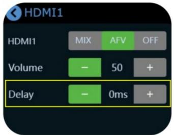
When the touch screen is in the main interface/ preview interface/Shortcut interface, the PGM audio volume can be adjusted by the toggle.
