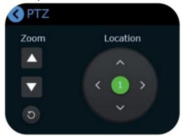
On the PTZ menu interface, when the PTZ function is enabled, the rotation angle of the PTZ can be adjusted by the joystick, and the focal length adjusted by the toggle.
