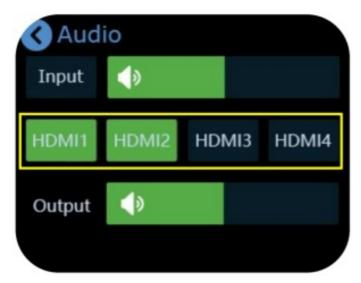
Turn on MIX to always add audio to PGM, Turn on AFV , the audio follows the video switch to perform a soft gradual transition when video is switched.
