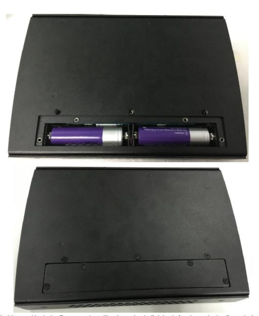
5. Install the holder, and lock the 7 screws, installing batteries is finished. As shown in the figure below
