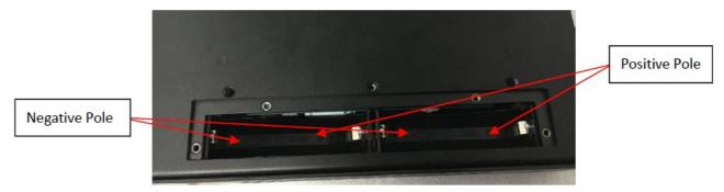
4. Install the 2 lithium ion batteries to the battery compartment one by one. Install the negative pole first, if install the positive pole first, maybe the battery can not be installed, or the battery compartment may be damaged. As shown in the figure below:
