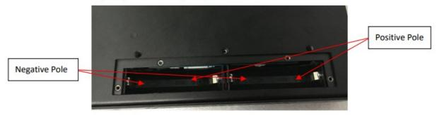
3. Install the 2 lithium ion batteries to the battery compartment one by one. Install the negative pole first, if install the positive pole first, maybe the battery can not be installed, or the battery compartment may be damaged. As shown in the figure below:
