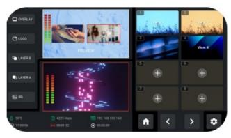
mini-edge allows user to save 10 presets in total. Rotate ENTER knob to View 1~10:
