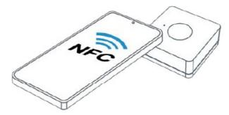
5. Basic information and settings of devices will be shown on ToolBox if it's recognized successfully. You can read and configure the device by tapping the Read/Write button on the App. In order to protect the security of devices, password validation is required when first configuration. The default password is 123456.
