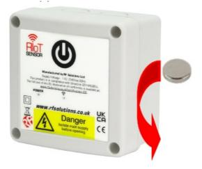
Briefly swipe a magnet along the enclosure to activate the internal reed switch.
