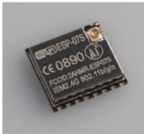
Figure 3 Top View of ESP-07s WiFi Module
