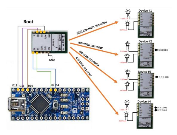
**Note:** The development board pins connected to RFLink-IO do not limit specific pins, you can also change them to other numbered pins.
