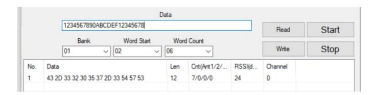
In the AnswerMode, select Stop, place a Tag on the Reader, select Write, then Start and Stop to read and confirm the Write was successful by viewing lower data display area which should now match that in the upper data display area. Replace with a new Tag, enter new Tag data and repeat to continue. You do not have to select Start, you can also select Read to read the Tag only once and output to the upper data display area.
