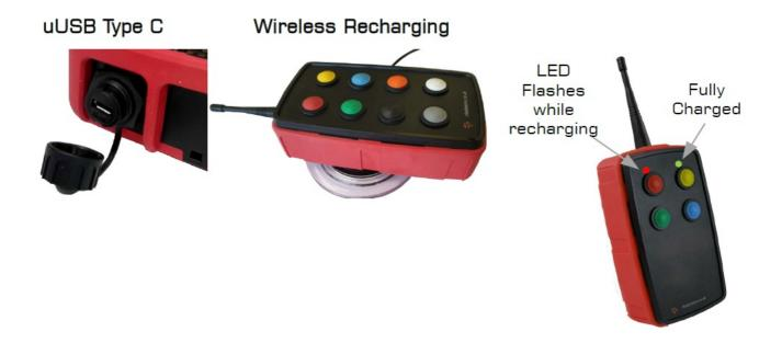
When Charging the Battery RED LED gives a slow Flash indicates charging is in prograess. When fully charged the GREEN LED is illuminated
