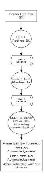
Acknowledg ement Feature provides the user with LED indication that the receiver has successfully received the transmitters signal. When activated the TAURUS Transmitter includes an acknowledgement request within each radio transmission.
