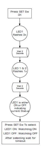
If enabled, TAURUS automatically transmits a background "watchdog" RF Signal approx. every ~45 secs, RF Solutions Receivers with a Watchdog feature will hold a Relay contact "ENERGISED" as long as Watchdog is regularly received confirming the transmitter is in range and the system is operating correctly. When using Watchdog it may be useful to incorporate a Power Switch to avoid premature battery discharge., A power switch can be incorporated if this is required please contact our Sales Dept.
