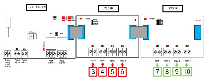
Input and Output modules can be added in any order by connecting with the Ribbon cables supplied. On initial Powerup EZTEXT automatically interrogates and configures additional modules. (all LEDS Flash). After approx. 60seconds the LEDs stop flashing to indicate the module is ready to use
