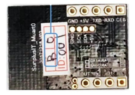
The MUART0-B Wireless UART Transmission Module is an easy-to-use module that instantly and painlessly upgrades wired UART to wireless UART transmission, in addition to being a set of 1/0 pins that allows you to eliminate the need for additional coding and hardware and have 10 switches that can be remotely controlled by each other to use.
