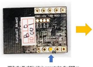
While the IN of this side is connected to the GND or tied LOW;
