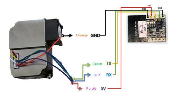
We can use a master board either Arduino or Raspberry Pi) and you can operate as normal wired UART mode to read the PM2.5 data from the G3. Congratulations! The G3 has been upgraded to have wireless transmission capabilities PM2.5 sensing module.
