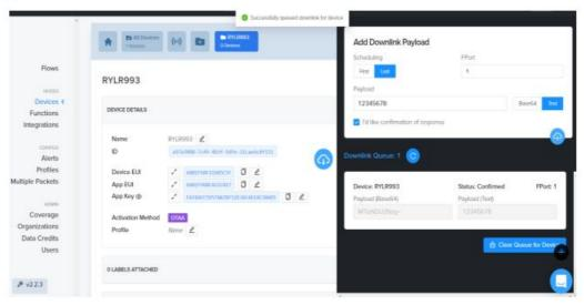
• Due to Helium Network can only download the data when RYLR993 is uploading the data, therefore it is needed to send "AT+SEND=1:1:31323334:", and RYLR993 will respond as below
