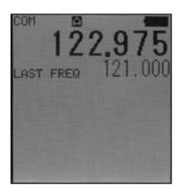
From the example above, the PJ2+ COM is receiving 122.975 MHz with the last frequency being 121.000 MHz. To manually enter a desired frequency such as 118.700 MHz, enter 1 1 8 7 0 0 using the numeric keypad. As each digit is entered, the flashing cursor moves to the next digit. Six digits may be required to select a frequency. The
