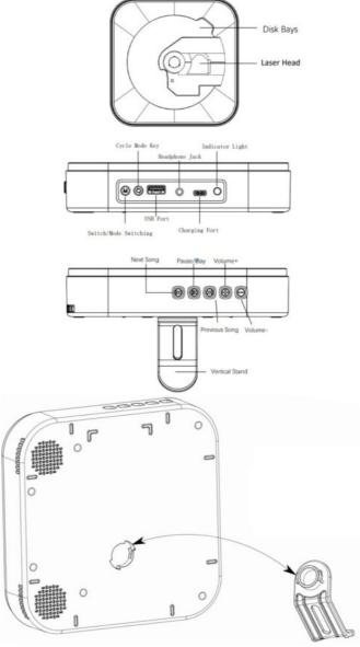
**Bracket Installation:** Align the bracket with the slot at the back of the machine, rotate it to the designated position, and then it can be used.
