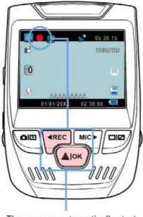
The camera automatically start recording when powered on
