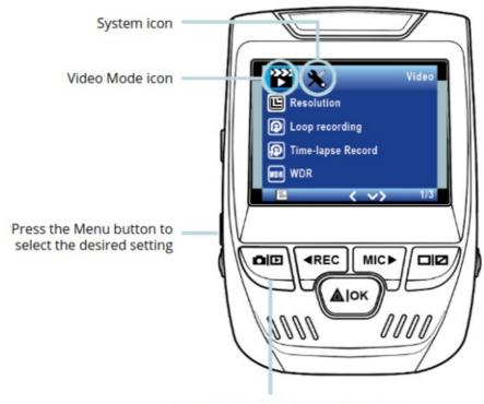
Press the Mode button and toggle to the desired Mode
