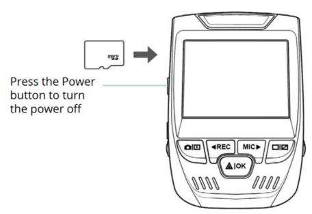
Step 3: Power the Camera and Format the Memory Card
