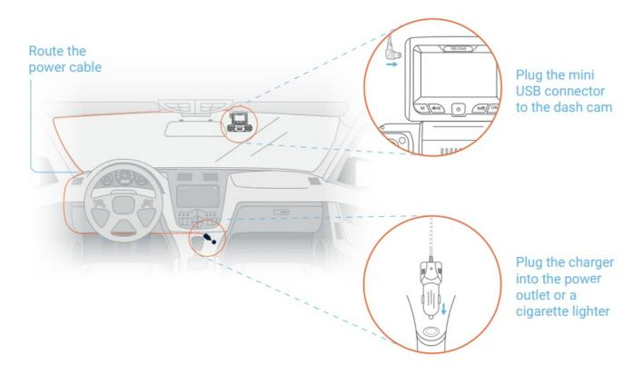
The camera will shut down after 3 seconds when it's disconnected from the power source and it should begin recording automatically the next time it is powered on. To ensure the S3 records to your memory card properly and without error, we strongly recommend you format the card within the camera when you're using the dash cam for the first time.
