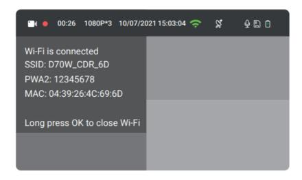
Open Settings on your phone (make sure that the Wi-Fi has turned on) and find the SSID in the network list, then enter the default password 12345678 to connect. Once it's connected, the Wi-Fi icon on the dash cam screen will turn to green.
