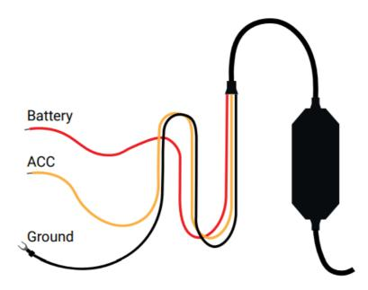
This feature will allow the dash cam to switch to parking mode automatically if the vehicle's engine turns off and switch back to the normal recording after the vehicle's engine turns on.
