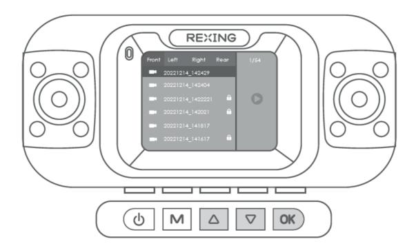
During playback, use the OK (pause), UP (rewind) and DOWN (fast forward) buttons to control the video playback. To playback a video using an SD card adapter, remove the memory card and insert it into an SD card adapter. Place the adapter in the computer. Then place the adapter into the computer. On the computer, navigate to device drive. Then select the video to playback.
