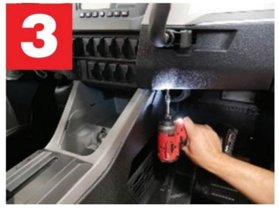
4. Flip the radio/intercom bracket backwards to use as a template and hold to dash. Mark (2) top mounting screw locations. Outline the left and right-side outer edges where the radio inserts. This helps to establish the upper surface material that needs to be left for the bracket to attach to.
