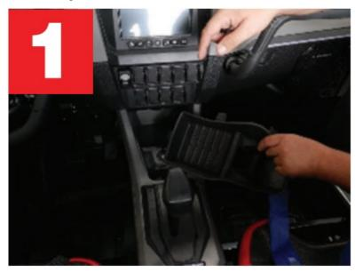
2. Remove automotive rivet from back wall of console storage pocket.
