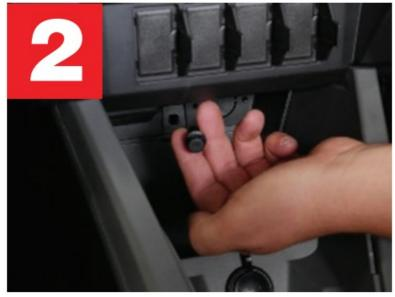
3. Remove (2) T30 Torx screws from underside of dash. One passenger side, one driver side. This will allow you to run cables down the center tunnel to the rear seats and battery.
