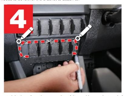
5. Draw two vertical lines straight down from the outer edge of the marking you just made for the radio. Outline the remainder of the storage pocket so you have a clear, cutting template.
