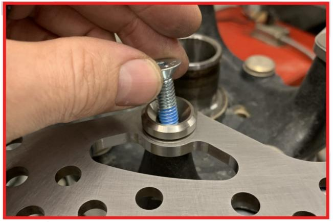
d. Reinstall the OEM hub with PM discs back onto the vehicle. Tighten the axle nut to 180 ft-lbs and install a new cotter pin.
