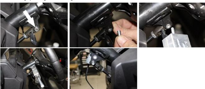
7. Install the Horn/Hazard Switch. Remove 1 of the switch plugs.
