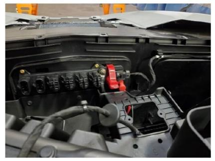
2. Mount the Control Module using the screw provided. Mount just to the side of one of the holes for Relays.
