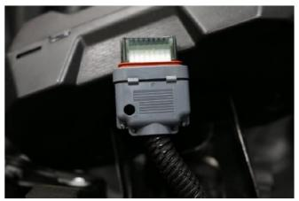
9. Remove Connector Lock – Using a small screwdriver push in on both sides at the white connector shown below and slide lock off.
