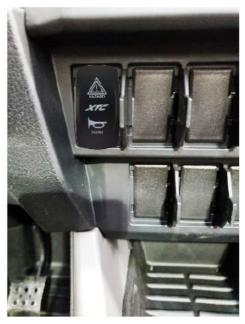
Run Switch Harness-Plug the Switch Harness into the Control Module, run Horn/Hazard connector through the rectangle switch cutout, and use included grease on switch terminals then connect the Switch and slide into the dash. NOTE: The switch cutouts are counter sunk, we have supplied 2 switch seals to be used as spacers to keep it raised out of the indent to keep it from getting stuck.
