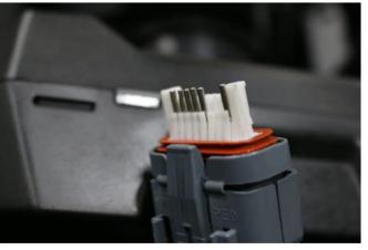
10. Remove Plugs – Using a pair of needle nose pliers remove the plugs from wire ports 6 and 7, insert the green wire terminal into 6 and the yellow wire terminal into port 7.
