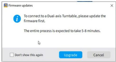
2. Click the "Upgrade" button, and the new firmware will be downloaded and installed automatically. Please follow the prompts to finish the firmware update. Once finished, the following window will pop up. And the 3D scanner will restart automatically.
