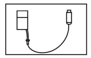
Align the charging head of the USB charging cable with the charging port of the battery and push together. NOTE: Charging input 5V, 200mA. (input current will directly affect charging time) The indicator light will stay constant when the battery is charging and tum off when the battery is fully charged. A full charge takes approximately 140 min.
