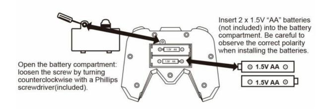
C lose the battery compartment :tighten the screw by turning clockwise with a Phillips screwdriver.
