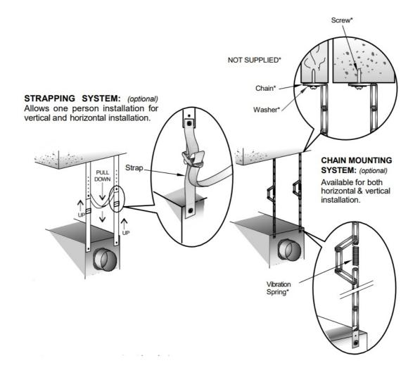
**Note:** After installation make sure the HRV/ERV is properly leveled. If not leveled correctly, then defrost will not perform effectively and/or unit may frost in winter.
