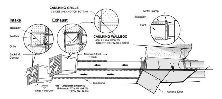
**Note**: Fresh air intake and supply duct must be totally insulated. Exhaust duct must be 5 feet insulated from the wall. In colder climate, it is recommended to insulate all exhaust
