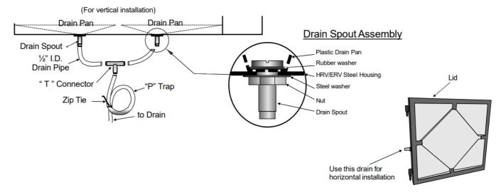
**Note**: For Horizontal installation, connect only 1 drain spout assembly on lid I door. cut one h" drain pipe and connect one end to the drain spout and the other end to the drain line. Don't forget to create a P-trap as shown above.
