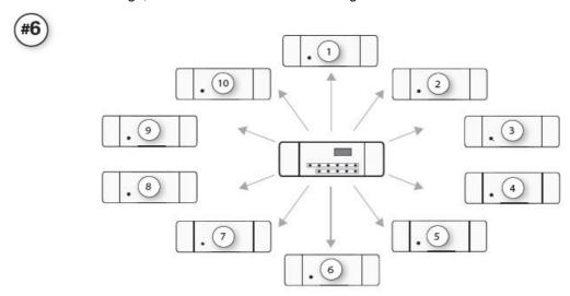
Each Parent Controller can control up to 10 Child Receivers
