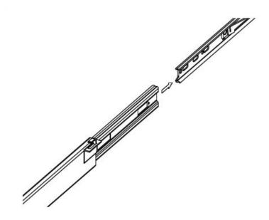
2. Lay both brackets on one side and attach the inner slide member to the brackets using the provided machine screws. Depending on your depth of closet will determine where your slides are mounted.
