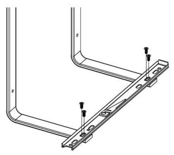
3. Once both inner slides member are attached to both sides you are now ready to attach the brackets to the underside of your shelf using the provided (4) wood screws.
