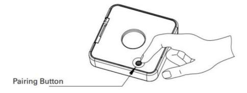
**Note:** Only one Receiver and one Dimmer can be paired. You cannot program for multiple Receivers and Dimmers.
