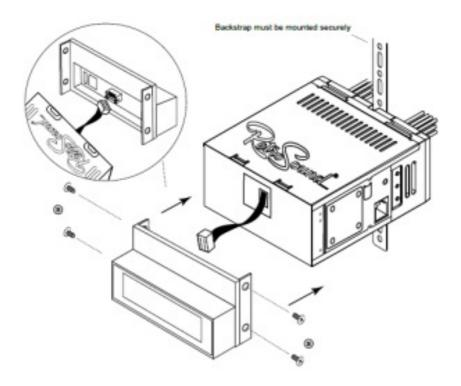
Plug the ribbon cable from the Radio Motor into the Radio Face. Attach the Radio Face to the Radio Motor with the four small screws.
