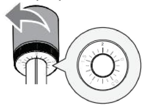
**Tip:** When setting the counterweight make sure you are turning the entire weight and not just the counterweight indicator ring.
