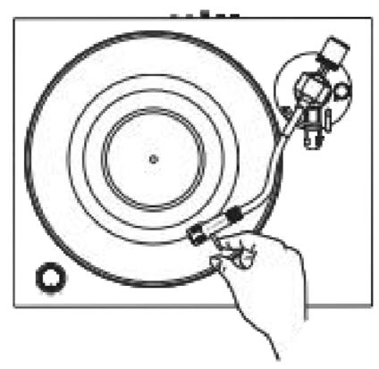
4. Hold the headshell and lower the cueing lever completely. Protect the stylus from touching the platter.
