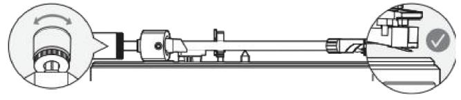
Tip: When balancing the tonearm make sure the cueing level is down.
