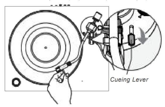
5. With the cueing lever now lowered, turn the entire counter weight until the tonearm is balanced and floating horizontally when headshell is released.
